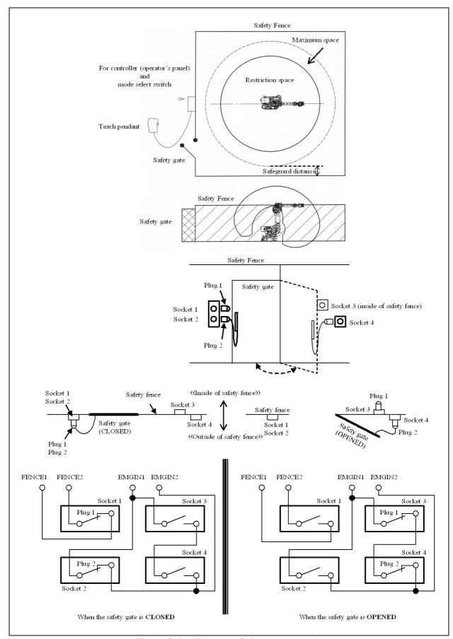
Fig. 4.9 Safety Fence and Safety Gate example
