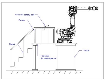
Fig. 3.2 Pedestal for maintenance
