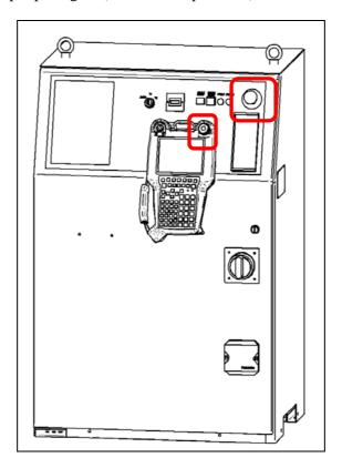
When the emergency stop button is pushed, the robot stops immediately (refer to Section 4.1 to 4.3). The external emergency stop input signal is input from peripheral devices.
